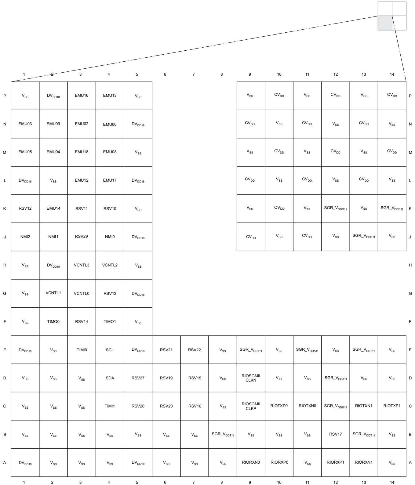
Figure 2-5. C6474 Pin Map (Bottom View) [Quadrant D]
