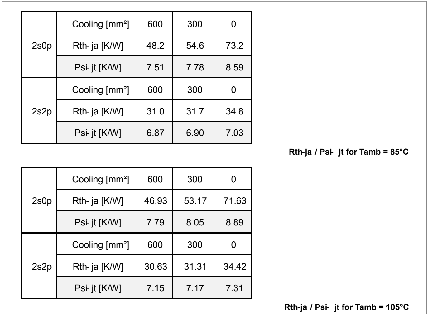
Figure 20 R_{thJA}/\Psi_{JT} results for both PCB designs
