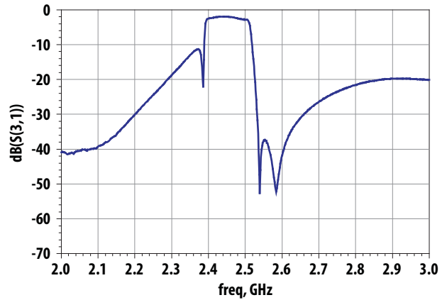
Figure 4. RX Path 2 – 3 GHz Frequency Response
