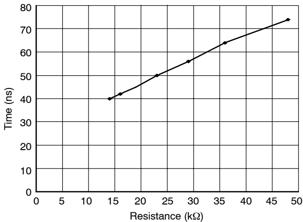
Figure 6. GATE Non-Overlap Time vs. DLYSET Resistance
